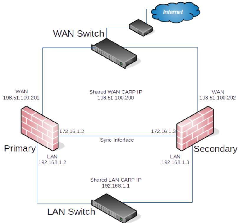
A total of **three ports on each device** will be used for the HA configuration. Each firewall will use a WAN port, a LAN port, and a third port between the two devices that will act as a sync interface to carry the heartbeat and sync the state information between the two devices.
